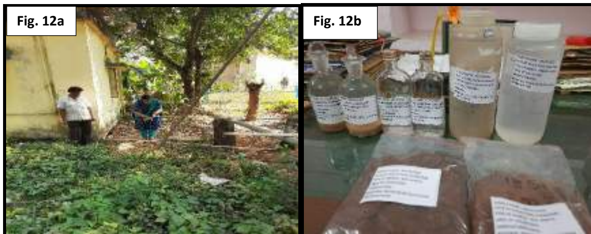
Fig.12a – Collection of Water Sample from the Borewell for Water Quality Testing, 12b- Soil and Water Samples Packed and Labelled as per the Instructions by the SPCB, Odisha INTEPRETATION OF WATER TEST RESULTS
