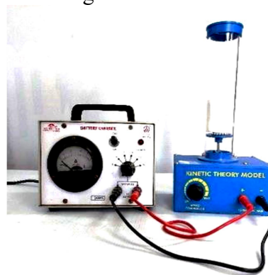
Fig.1: Random motion of steel balls depicting Kinetic Theory of gas molecules
