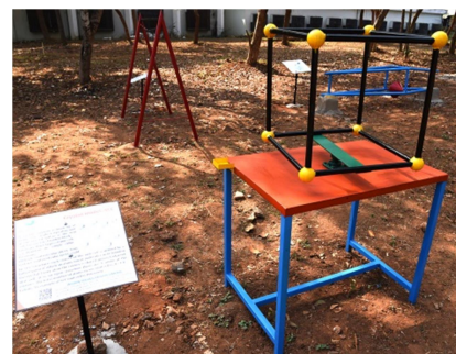
(Demonstration of simple cubic crystal structure)
