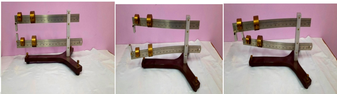
Fig.6 : Coupled oscillation of two metallic vibrators producing beat
