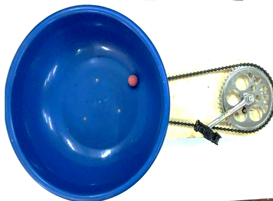
Fig.17 : Rotation of a ball in a tub due to centripetal force
