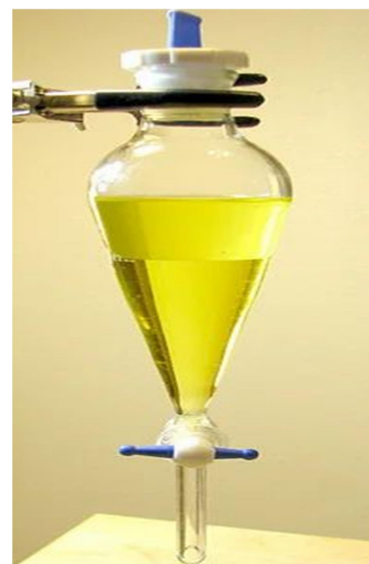
Fig.41: Separation funnel showing two different layers if immiscible liquids
